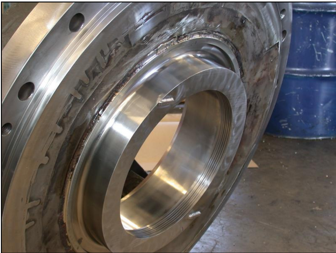
MST #08: MST's Modular Stuffing Box Upgrade Installing into a Small Head
