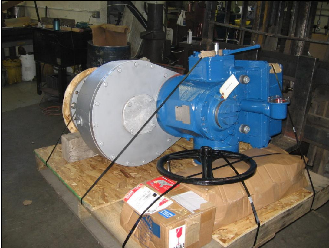
MST #06: Restored Gearbox & Actuator Assembly
