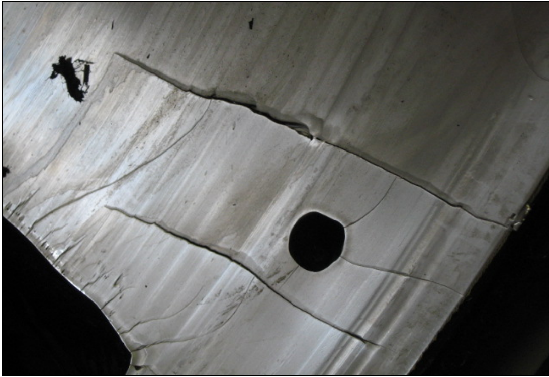
MST #13: Severe Cracks From Poor Weld Preps (Prior Vendor Unknown)
