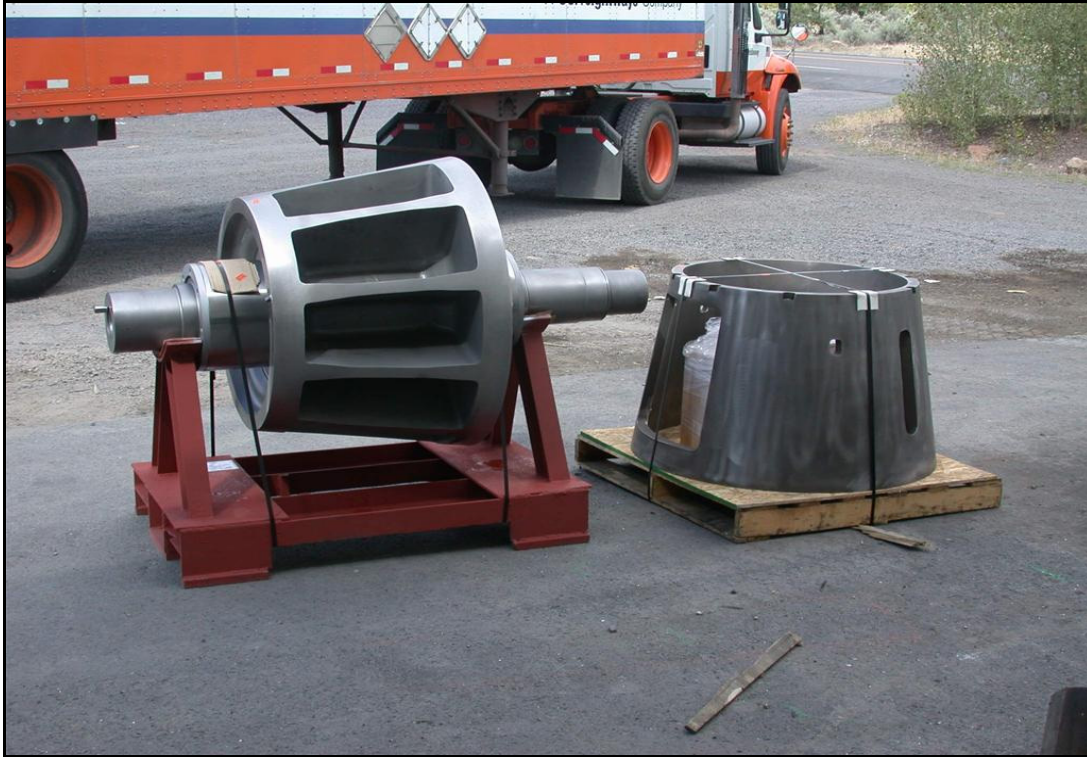
MST #05: Model 69 /451-18" Rotor & Liner High Pressure for Cotton Linters
