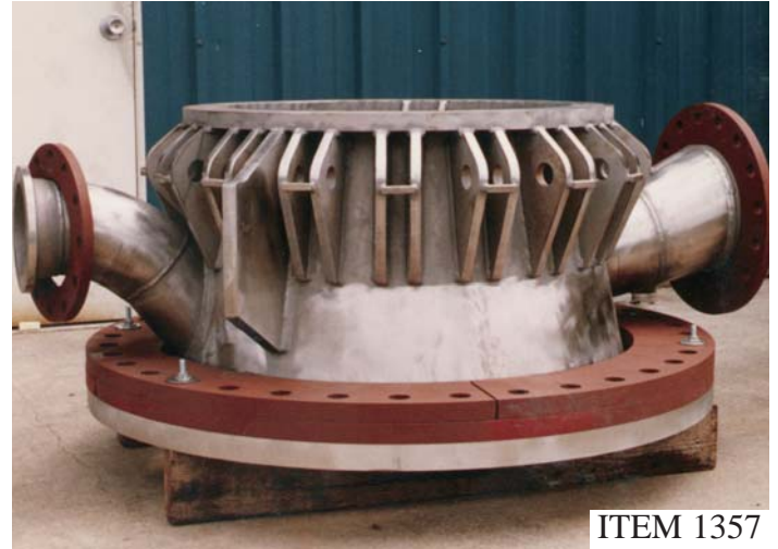
HIGH ALLOY T317 SS BATCH DIGESTER CHIP PACKERS. THESE UNITS (EIGHT TOTAL) WERE MANUFACTURED BY MST TO REPLACE FAILED OEM UNITS CODE CONSTRUCTION
