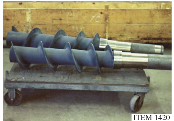
TWIN FEED SCREW RESTORATION SCREW SECTION COATED WITH SPECIAL WEAR RESISTANT CERAMIC
