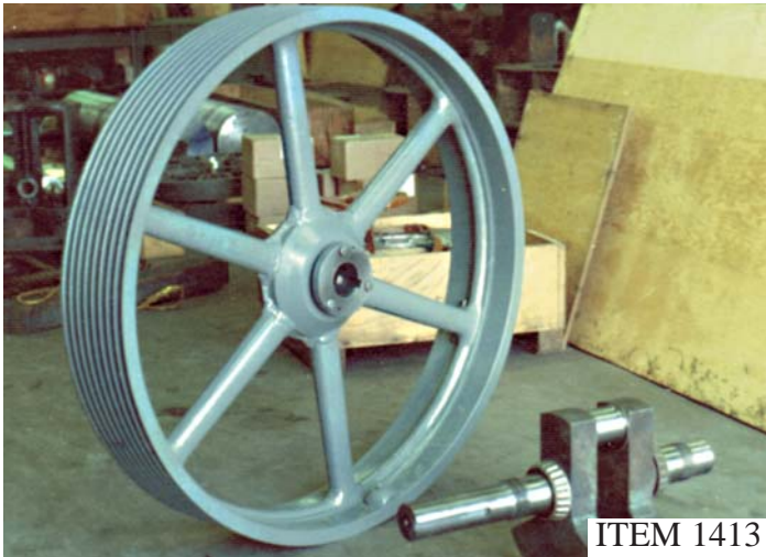
COMPRESSOR CRANK AND PULLEY RESTORATION
