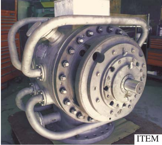
MST CUSTOM 30" HIGH PRESSURE ROTARY VALVE
