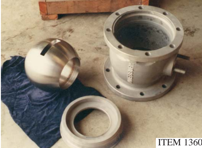
RESTORED AND ALLOY UPGRADE FOR BALL VALVE ASSEMBLY
