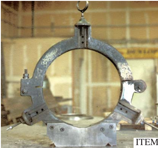
WELD RESTORE BROKEN LATHE STEADY REST
