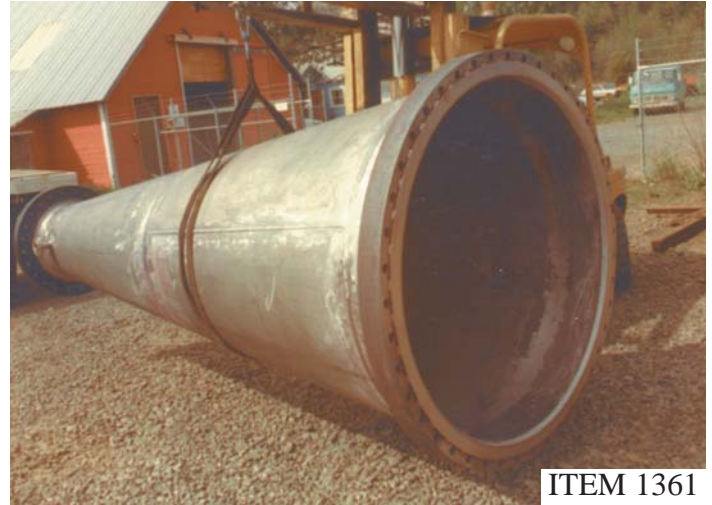
SUPER ALLOY FABRICATION OF TRANSITION VESSEL FOR MOUNTING BAUER HIGH PRESSURE ROTARY VALVE
