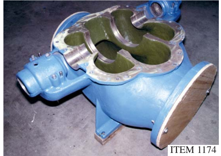
FAN PUMP HOUSING RESTORED THEN LINED WITH SPECIAL EPOXY PROTECTION SYSTEM
