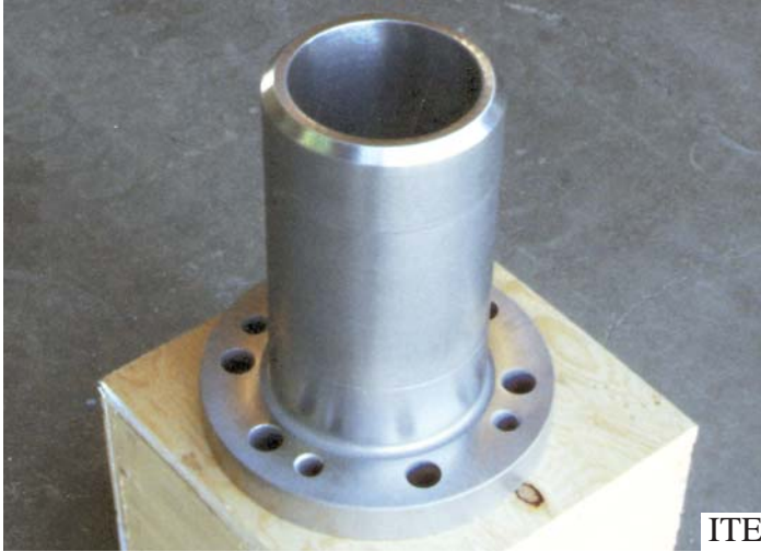
CUSTOM 440C - SPECIAL PROCESS AND HEAT TREATMENT NON LUBRICATED SUBMERGED SHAFT BEARING BUSHING
