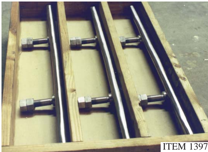
REMANUFACTURE SPECIALTY SEPARATOR ROTOR WITH INTEGRAL FOIL BARS
