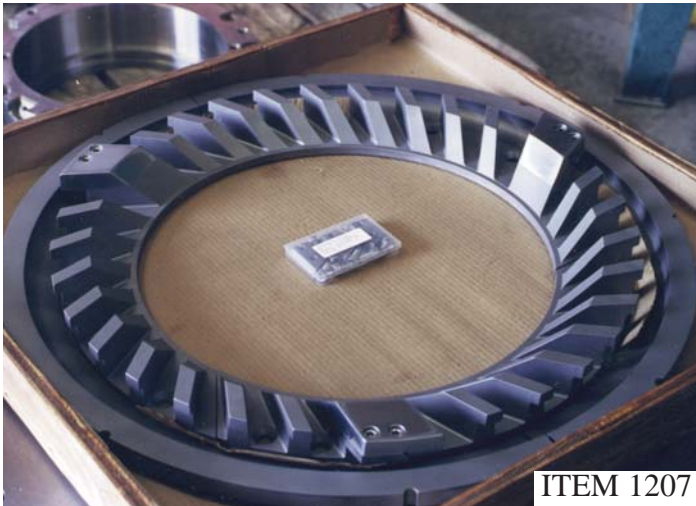
SHREDDER ANVIL AND ROTOR MANUFACTURED NEW, BY MST
