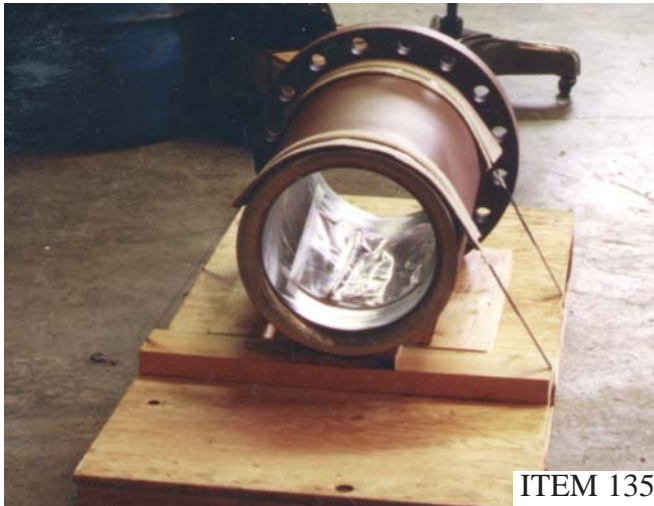
NEW INTERNAL LOAD SENSOR HOUSING FOR SPROUT BAUER REFINER
