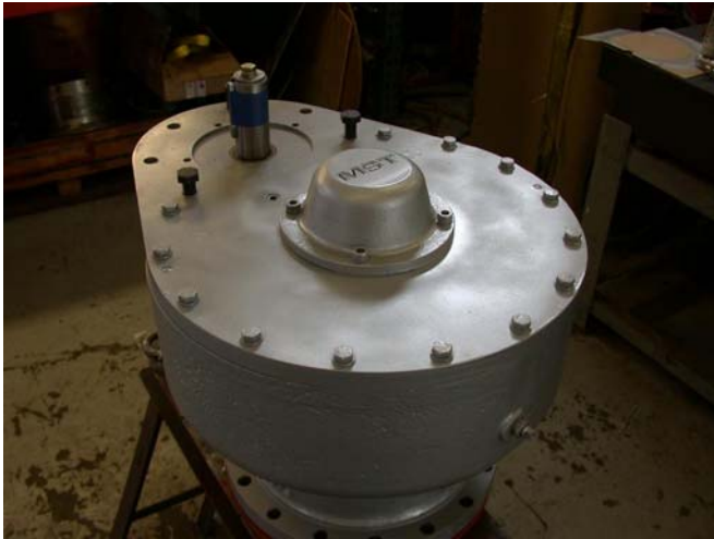
Limiter Gearbox Restoration
