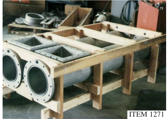
REFINER IN-FEED LOAD SENSOR HOUSINGS RESTORATION CODE WELDED
