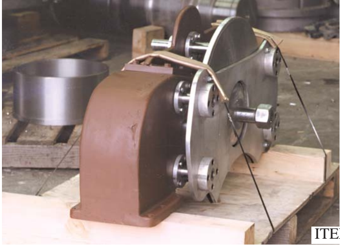
SPECIAL DOUBLE DISC GRINDER GRINDING AUTOMATIC FEED ATTACHMENT - DESIGNED AND MANUFACTURED BY MST
