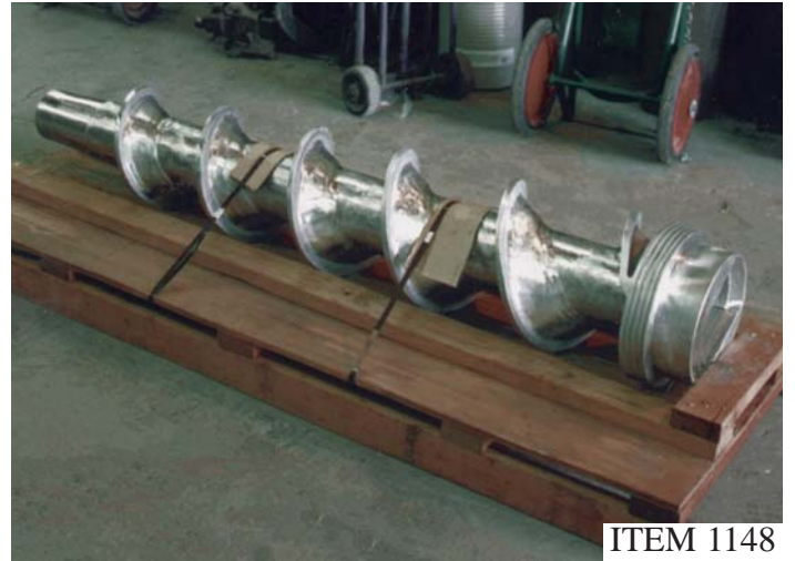
PLUG SCREW FEEDER SCREW RESTORATION
