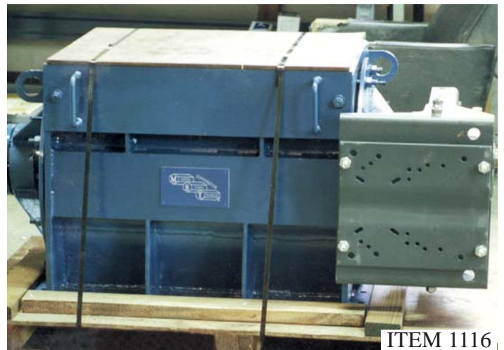
CUSTOM AIR LOCK FEEDER WITH INTEGRAL DRIVE SYSTEM AND COMPENSATOR THRUST
