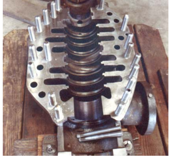
SIX STAGE FEED WATER PUMP HOUSING WELD RESTORED BY MST AFTER CATASTROPHIC FAILURE MACHINED AND LINE BORED BY MST
