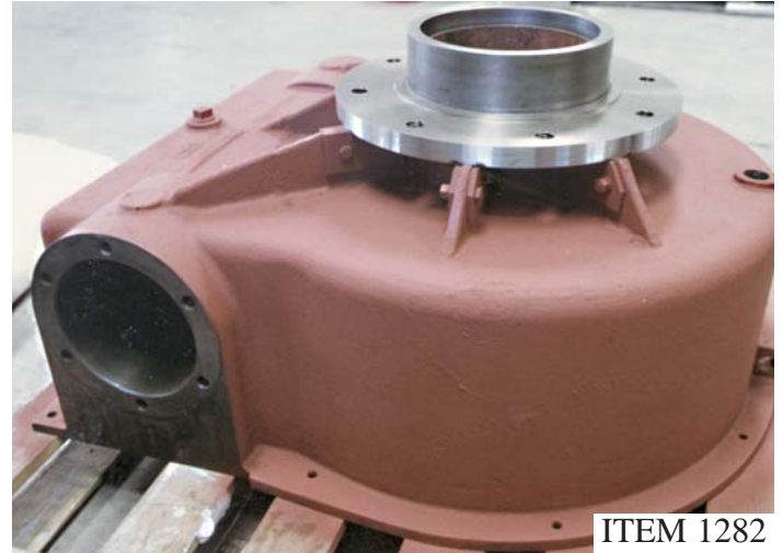
GEAR HOUSING-MODIFIED TO TAKE SS FITTING SHOWN
