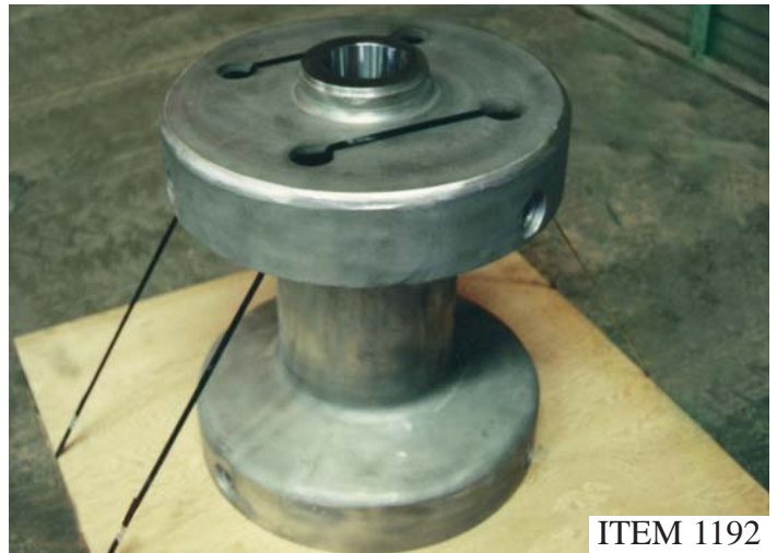
ROUND SCREEN FOIL BAR ROTOR RESTORATION AND UPGRADE
