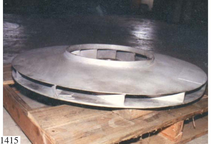
SUPER ALLOY FAN SHOWN AFTER RESTORATION
