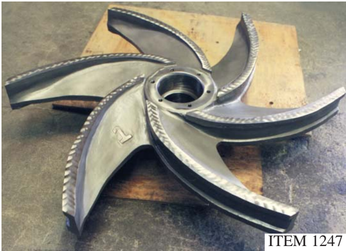
PULPER ROTOR IN RECYCLING SYSTEM UPGRADED FOR 200 EXTRA HORSEPOWER OPERATION
