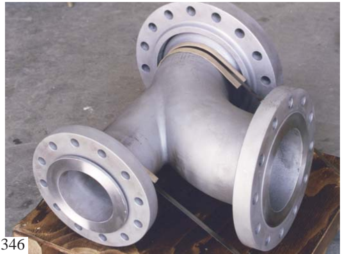
SPECIAL SS BLOW LINE DIGESTER FITTING LONG LIFE DESIGN, REDESIGNED TO TAKE SPECIAL SLIP RING FLANGE FOR FIELD ALIGNMENT ISSUES
