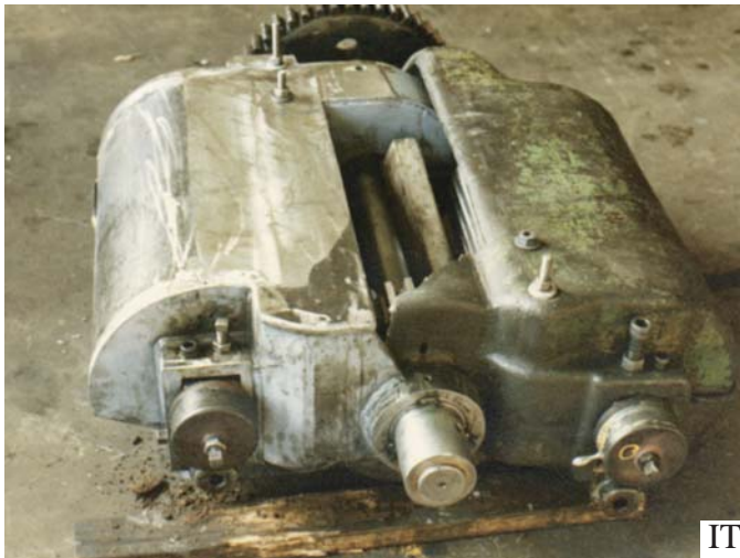
SAWMILL APPLICATION - OBSOLETE EQUIPMENT RESTORATION DESIGNED AND FABRICATED - NEW HOUSING SECTION TO REPLACE FAILED CAST IRON - REVERSE ENGINEERED BY MST
