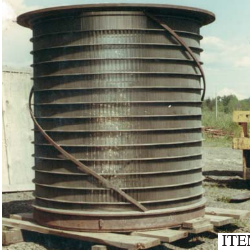
KAMYR® TOP SEPARATOR SLOTTED BASKET RESTORATION
