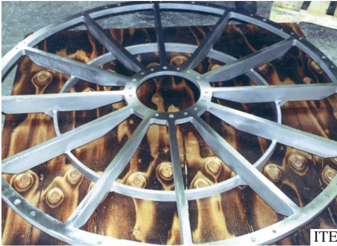
EXTRACTION PLATE FRAME RESTORATION
