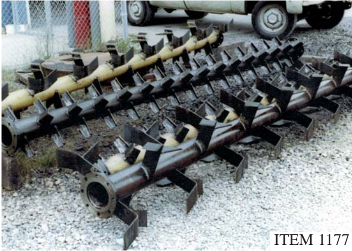
PULP DRYER SHREDDER ROLLS REVERSE ENGINEERED AND MANUFACTURED NEW BY MST
