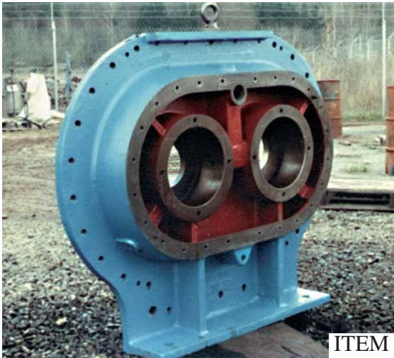
RESTORED BLOWER END BELL, READY FOR ASSEMBLY
