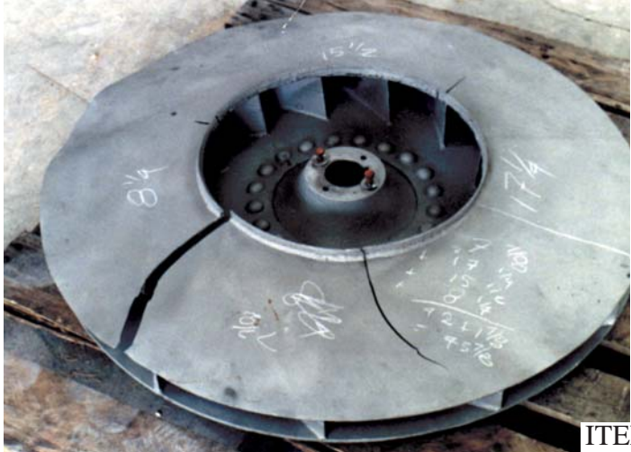
SUPER ALLOY FAN SHOWN BEFORE RESTORATION
