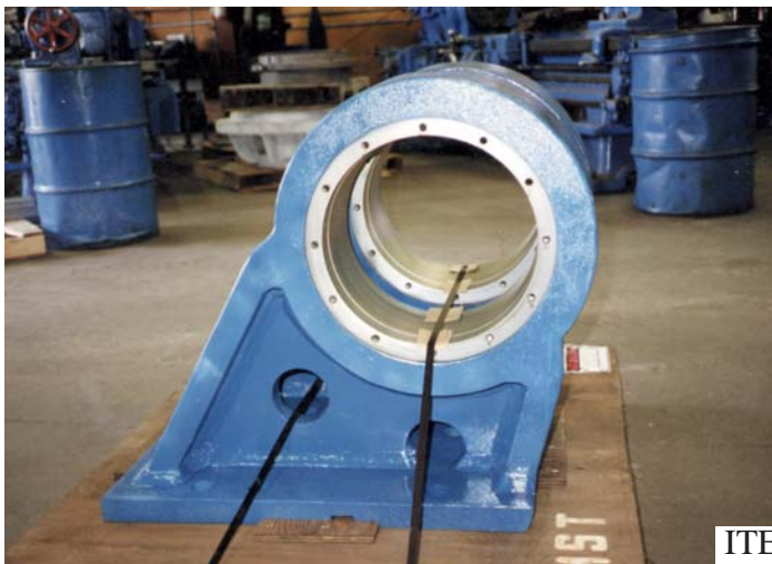
PAPER MILL ROLL SPECIAL BEARING MOUNT HOUSING SYSTEM REMANUFACTURED
