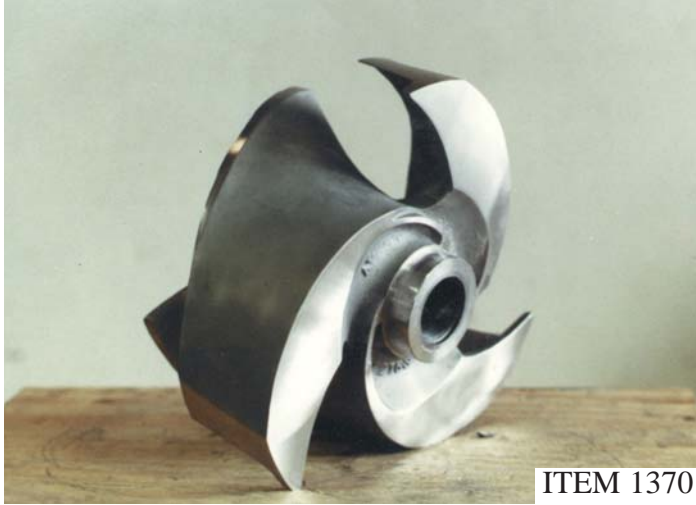
VARIOUS PUMP IMPELLER RESTORATION
