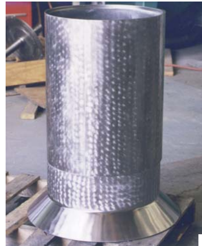
BELOIT LOBBED ROTOR AND UPPER WEIR MANUFACTURE NEW BY MST
