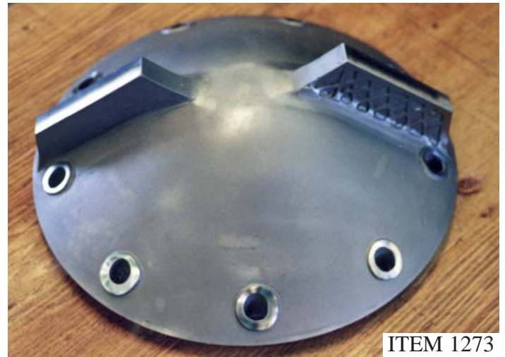
PULPER ROTOR CENTER HUB SECTION RESTORATION AND BAR REPLACEMENT
