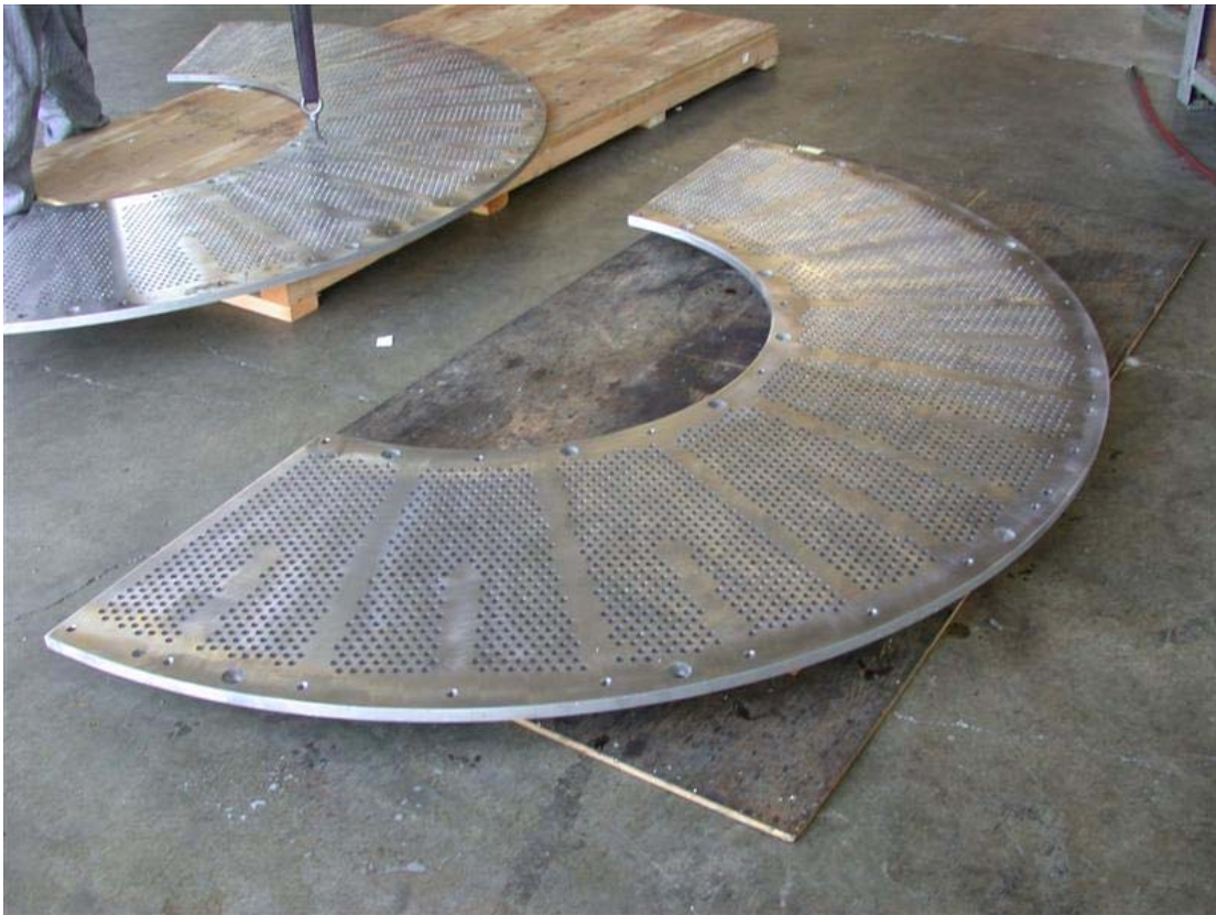
#1439 VSAP-100 Voith 98" Diameter Extraction Plates Mfg New by MST CNC machine
