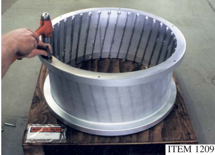
RESTORATION AND BAR REPLACEMENT OF SEPARATOR SCREEN
