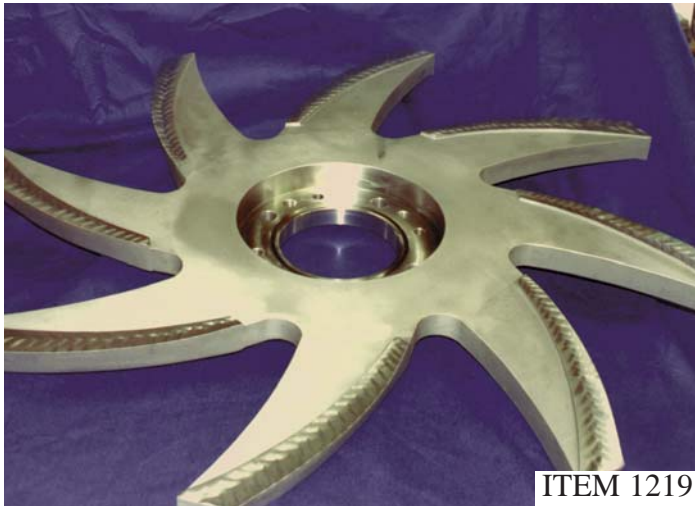
MANUFACTURE AND UPGRADE SEPARATOR ROTOR
