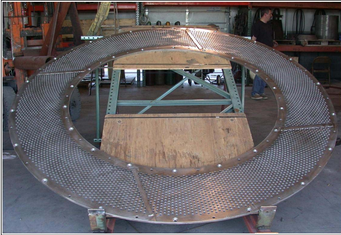
106" DIAMETER EXTRACTION PLATE FOR SECONDARY FIBER /OCC RESTORE OR MANUFACTURE NEW
